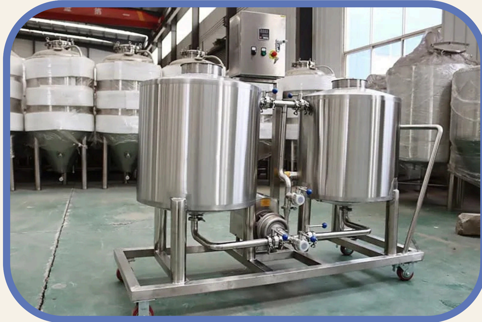
CIP (Cleaning In Place)
